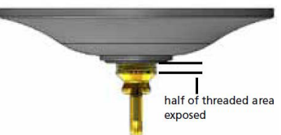
Drawing 2 – Canopy Adjustment
