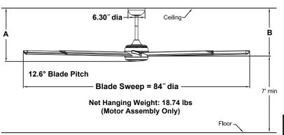
Fan must be attached to a securely anchored electrical junction box capable of withstanding a load of at least 35 lbs.
